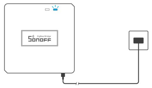
Power the device through a Micro USB cable. After powering on, the device will enter the Bluetooth Pairing Mode during the first use. The Wi-Fi LED indicator changes in a cycle of two short and one long flash and release.
