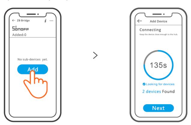
Make the sub-devices enter the pairing mode, tap "Add" icon on the Zigbee Bridge interface, then wait it to find the sub-devices and pair.
