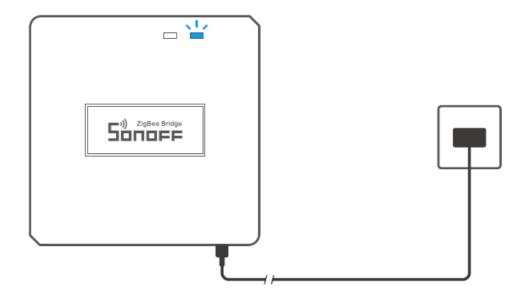
Power the device through Micro USB cable. After powering on. the device will enter the Bluetooth Pairing Mode during the first use. The Wi-Fi LED indicator changes in a cycle of two short and one long flash and release. The device will exit the Bluetooth Pairing Mode if not paired within 3mins. If you want to enter this mode, please long press pairing button for about 5s until the Wi-Fi LED indicator changes in a cycle of two short and one long flash and release.
