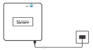
The device will exit the Pairing Mode if not paired within 3mins. If you want to enter this mode, please long press pairing button for about 5s until the Wi-Fi LED indicator changes in a cycle of two short and one long flash and release.
