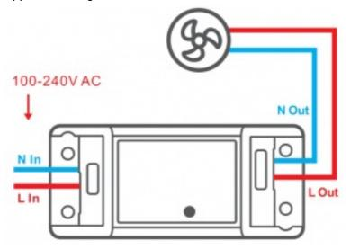
• Make sure the neutral wire and live wire connection is correct.
