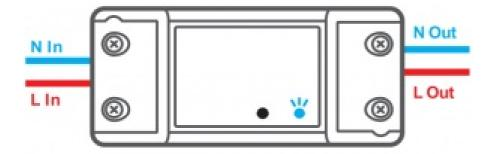
The device will exit the quick pairing mode (Touch) if Wi-Fi connection is not successful within 3mins. If you want to enter this mode, please long press the manual button for about 5s until the Wi-Fi LED indicator changes in a cycle of two short and one long flash and release.
