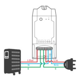
Make sure the neutral wire and live wire connection are correct.
