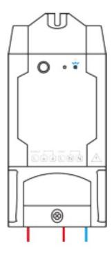
After powering on, the device will enter the quick pairing mode (Touch) during the first use. The Wi-Fi LED indicator changes in a cycle of two short and one long flash and release.
