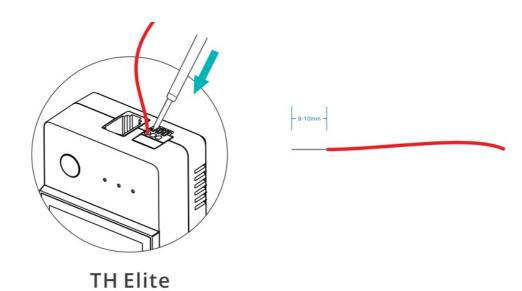
Press the white button on the top of the wire connecting hole to insert the wire corresponding, then release.
