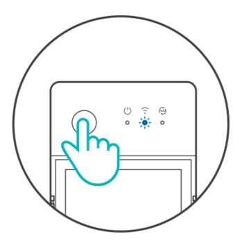
The device will exit the Bluetooth Pairing Mode if not paired within 3mins. If you want to enter this mode, please long press button for about 5s until the Wi-Fi LED indicator changes in a cycle of two short and one long flash and release.
