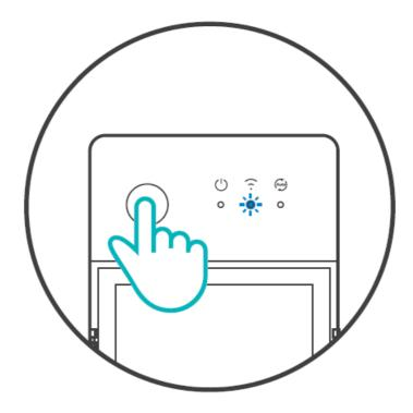
The device will exit the Pairing Mode if not paired within 3mins. If you want to enter this mode, please long press button for about 5s until the Wi-Fi LED indicator changes in a cycle of two short and one long flash and release.
