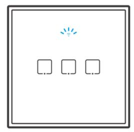
After powering on, the device will enter the quick pairing mode (Touch) during the first use. The Wi-Fi LED indicator changes in a cycle of two short and one long flash and release. • The device will exit the quick pairing mode (Touch) if not paired within 3mins. If you want to enter this mode, please long press any configuration
