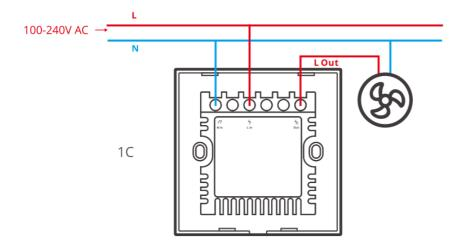
Make sure all wires are connected correctly.
