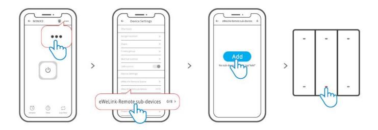
Enter the setting interface of "eWeLink-Remote" gateway, click "eWeLink-Remote sub-devices" and "add", then trigger any button on R5 to add successfully.
