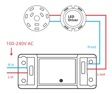
Make sure the neutral wire and live wire connection is correct.
