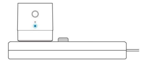
Powering on, the device will enter the quick pairing mode (Touch) during the first use. The Wi-Fi indicator flashes quickly.
