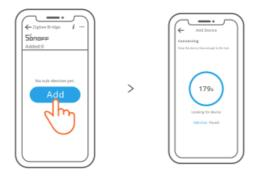
On the Zigbee gateway main page of the eWeLink App, click "Add" sub-devices and wait for the addition process to complete. If the device is failed to be added, please move the device closer to the Bridge and add it again
