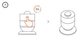
The device will exit the pairing mode when it doesn't be paired to Zigbee gateway successfully within 3mins. If you want to access the pairing mode again, press and hold the device pairing button for 5s until the LED indicator "flashes slowly" If the device is the No battery version, please install the battery (CR2477) to power on the device.
