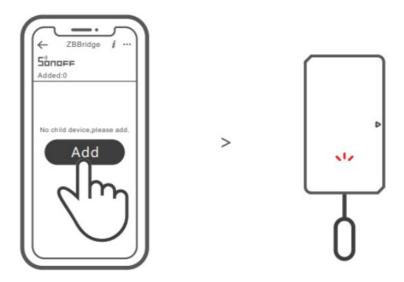
Access eWeLink APP, select the Bridge that you want to connect and tap "Add" to add a sub-device. Then long press reset button on the device for 5s until the LED indicator flashes three times, which means the device has entered the pairing mode, and be patient until pairing completes.
