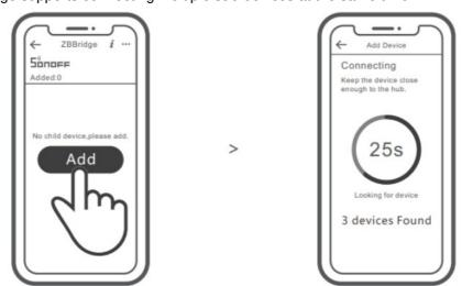
Power the Bridge on, access the Bridge page in the eWeLink APP, and tap "Add". Then set the sub-device to be paired to the pairing mode and be patient until the pairing completes.
