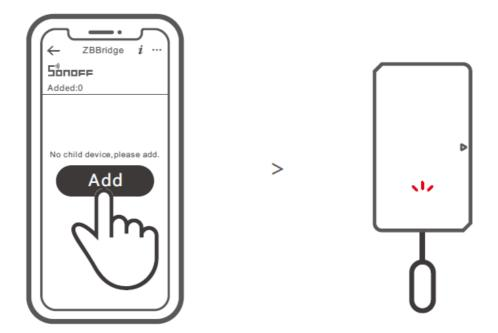
Access eWeLink APP, select the Bridge that you want to connect, and tap "Add" to add a sub-device. Then long press the reset button on the device for 5s until the LED indicator flashes three times, which means the device has entered the pairing mode, and be patient until pairing completes.
