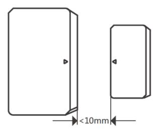
Make sure the installation gap is less than 10mm when the door or window is closed. The device's weight is less than 1 kg. An installation height of less than 2 m is recommended.
