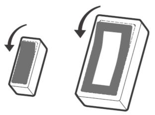
2. Try to align the marked line on the magnet with that on the transmitter during installation.
