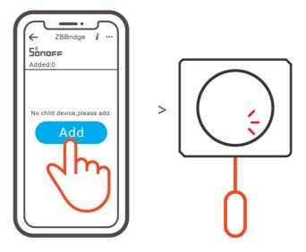
Access eWeLink APP, select the Bridge that you want to connect and tap "Add" to add a sub-device. Then long-press the reset button on the device for 5s until the LED indicator flashes three times, which means the device has entered the pairing mode, and be patient until pairing completes.
