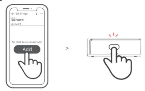
Access eWeLink App, select the Bridge that you want to connect, and tap "Add" to add a sub-device. Then long-press the reset button on the device for 5s until the LED indicator flashes slowly, which means the device has entered the pairing mode, and be patient until pairing completes.
