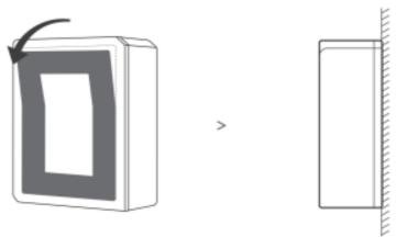
Do not install on the metal surface, otherwise, it will affect the wireless communication distance.
