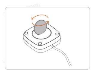
Use a coin to twist and remove the battery cover.
