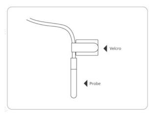
Tear off the Velcro adhesive and fix the probe to the location where detection is required (for example: in the refrigerator, next to the swimming pool and so on).
