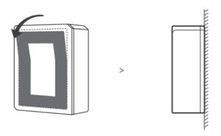
▲ Do not install on the metal surface, otherwise it will affect the wireless communication distance. Installation methods 10 SONOFF TECHNOLOGIES CO., LTD. English The device weight is less than 1 kg.
