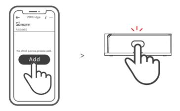
Access eWeLink APP, select the Bridge that you want to connect, and tap "Add" to add a sub-device. Then long press reset button on the device for 5s until the LED indicator flashes three times, which means the device has entered the pairing mode, and be patient until pairing completes.
