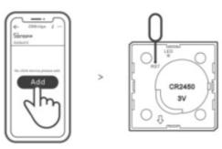
Access eWeLink APP, select the Bridge that you want to connect, and tap "Add" to add a sub-device. Then long press "RST" reset button on the device for 5s until the LED indicator flashes three times, which means the device has entered the pairing mode, and be patient until pairing completes. If the addition failed, move the sub-device closer to the Bridge and try again.
