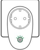
After power on the device, it will enter the FFS pairing mode defaulted and the Zigbee LED indicator will flash slowly".
