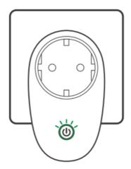
After powering on, the device will enter the pairing mode defaulted during the first use and the Zigbee LED indicator will "flash slowly".
