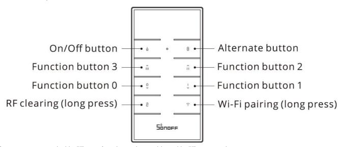
Buttons are created with different functions when pairing with different products.
