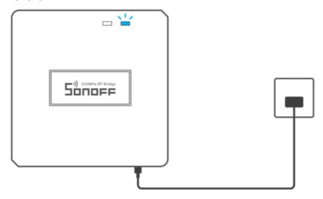
Use the Micro USB cable to power the device, After powering on, the device will enter the quick pairing mode during the first use. The Wi-Fi LED indicator changes in a cycle of two short and one long flash.
