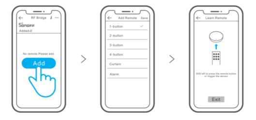
Click "+", select the type of remote control. The device enters the learning mode when you hear a beep from it, and then press the 433MHz remote control or trigger the sensor, and you will hear two beeps to complete the learning process.
