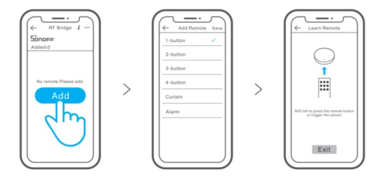
Tap "+" and select the remote controller type, then a "Beep" indicates that the device enters quick pairing mode. Proceed to operate on the sub-device to pair and "Beep Beep" indicates that the pairing is successful.
