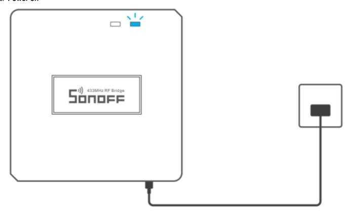
After powering on, the device will enter the quick pairing mode (Touch) during the first use. The Wi-Fi LED indicator changes in a cycle of two short and one long flash.
