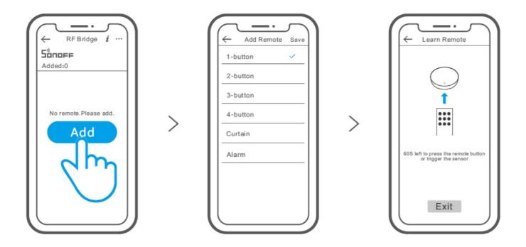
Tap "+" and select the remote controller type, then a "Beep" indicates that the device enter quick pairing mode. Proceed to operate on the sub-device to pair and "Beep Beep" indicates that the pairing is successful.
