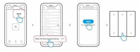
Enter the setting interface of the "eWelink-Remote" gateway, click "eWelink-Remote sub-devices" and "add", then trigger any button on RS to add successfully.
