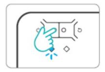
The device will exit the quick pairing mode (Touch) if not paired within 3mins. If you want to enter this mode, please long press the pairing button of about 5s until the Wi-Fi LED indicator changes in a cycle of two short and one long flash and release.
