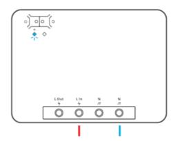
After powering on, the device will enter the quick pairing mode (Touch) during the first use. The W-FI LED indicator changes in a cycle of two short and one long flash and release.
