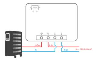
Make sure all wires are connected correctly.
