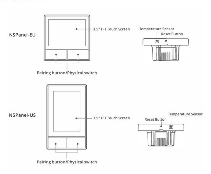
The device weight is less than 1 kg. The installation height of less than 2 m is recommended.
