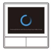
After powering on, the device will enter the Bluetooth Pairing Mode during the first use. The screen status is shown in the above image.
