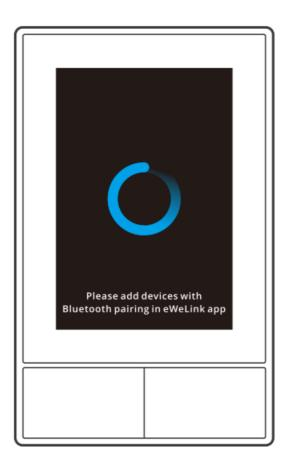
After powering on, the device will enter the Bluetooth Pairing Mode during the first use. The screen status is shown in the above image.
