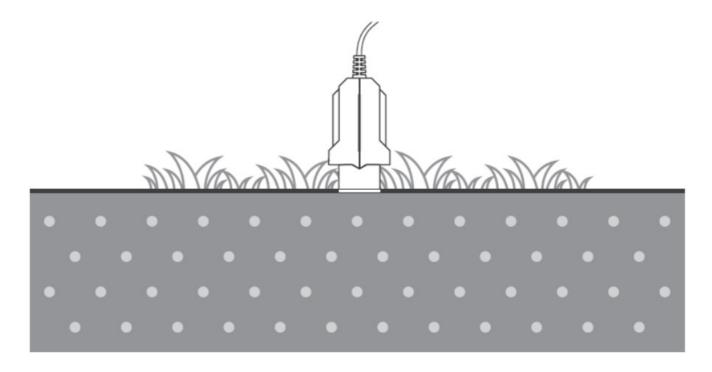
The sensor can be extended with the extension cable (AL560\*2), up to 10M. (AL560 is not included in the package, please order separately).
