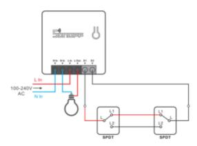
(!) Make sure the neutral wire and live wire connection is correct.
