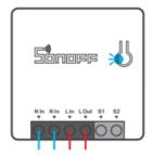
After powering on, the device will enter the quick pairing mode (Touch) during the first use. The Wi-Fi LED indicator changes in a cycle of two short and one long flash and release.
