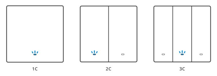
After powering on, the device will enter the Pairing Mode during the first use. The Wi-Fi LED indicator changes in a cycle of two short and one long flash and release.
