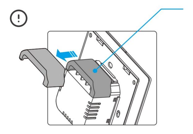
① When the wall-mounting box is made of plastic and the size is small, the protective cover can be omitted .
