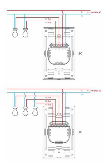
Make sure all wires are connected correctly.
