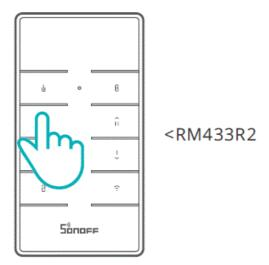
After powering on iFan04, press any button on the controller until the buzzer makes a "beep" sound within 5s, then all the buttons are learned successfully. If you do not operate any step within 5s, power the device on again and repeat the above operation.
