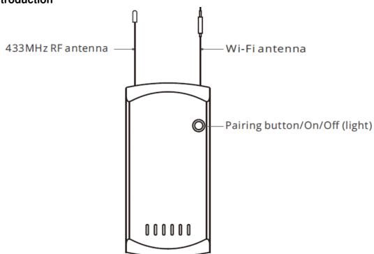
The device weight is less than 1 kg. The installation height of less than 2 m is recommended.
