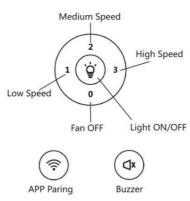
First, you'll need to install the battery. You will need a slotted screwdriver to open the battery cover on the Remote's back. You can use RF Remote to control the fan and light, change the fan speed(1/2/3), close the buzzer if you don't want to hear the beep sound of every operation.
