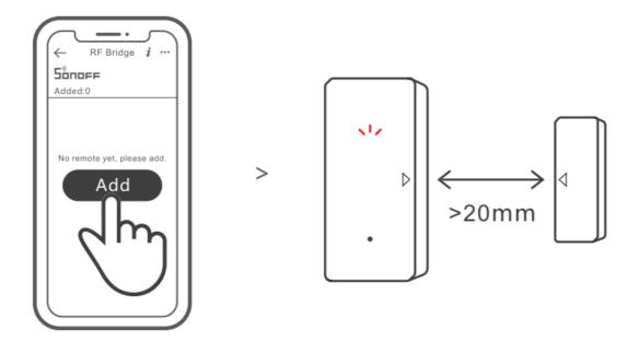
Access the eWeLinkAPP and select the Bridge, tap "Add" to select the alarm, and a "Beep" means the Bridge enters the pairing mode. Then separate the magnet for more than 20 mm from the transmitter until the LED indicator stays on for 1 to 2s, and the pairing is complete when you hear "Beep Beep".
