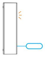
Long press the pairing button on the transmitter for 5s with the eject pin until the LED indicator flashes, then the device enters the pairing mode.
