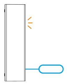
Long press the pairing button on the transmitter for 5s with the eject pin until the LED indicator flashes, then the device enters the pairing mode.
