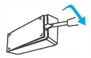
• Remove the back cover of the transmitter
