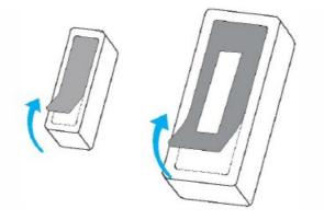
• Tear off the protective film of the 3M adhesive.
