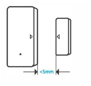
• Make sure the installation gap is less than 5mm when the door or the window is closed.
