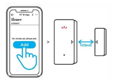
Access the eWeLinkAPP and select the Bridge, tap "Add" to select the alarm, and a "Beep" means the Bridge enters the pairing mode. Then separate the magnet for more than 20 mm from the transmitter until the LED indicator stays on for 1 to 2s, and the pairing is complete when you hear "Beep Beep".
