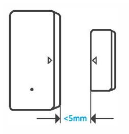
• Try to align the mark line on the magnet with that on the transmitter during installation
