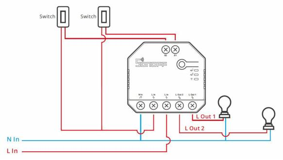
2. Connect SPDT switches in the edge mode to reach double two-way control
