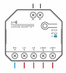
After powering on, the device will enter the bluetooth pairing mode during the first use. The Wi-Fi LED indicator changes in a cycle of two short and one long flash and release. The device will exit the bluetooth pairing mode if not paired within 3mins. If you want to enter this mode, please long press the manual button for about 5s until the Wi-Fi LED indicator changes in a cycle of two short and one long flash and release.
