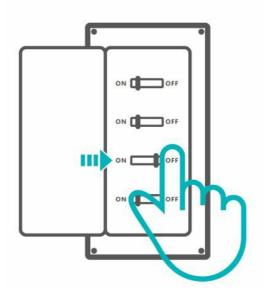
To avoid electric shocks, please consult the dealer or a qualified professional for help when installing and repairing! Do not wire when power is on.
