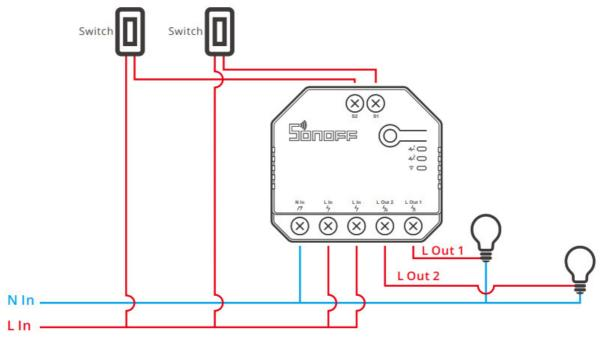
2. Connect SPDT switches in the edge mode to reach double two-way control:
