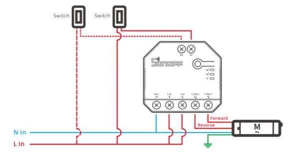
Connect to S1 or S2 for smart control of connected devices; connect to S1 and S2 for two-way smart control.
