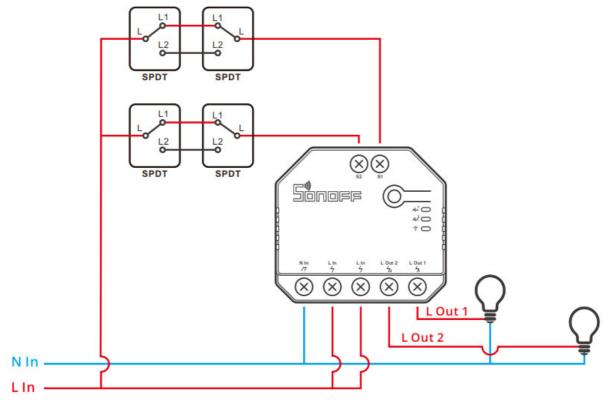
3. Connect dry contact sensors in the following mode:
