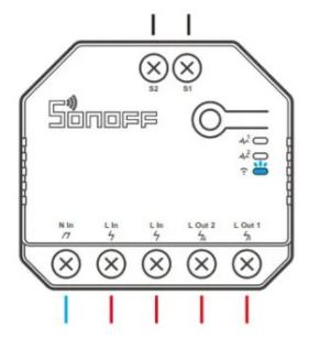
After powering on, the device will enter the Bluetooth pairing mode during the first use. The Wi-Fi LED indicator changes in a cycle of two short and one long flash and release.
