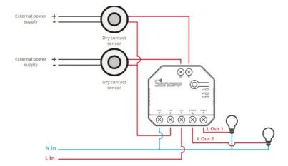
3. Connect dry contact sensors in the following mode:
