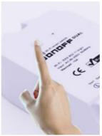
2. Press the pairing button for 7 seconds until the green LED blinks like below: the LED blinks 3 times and on repeatedly .
