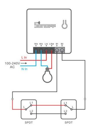
S1/S2 can connect with the rocker light switch or doesn't connect. To ensure safety, do not connect the neutral wire and live wire lo it.
