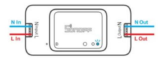
After powering on, the device will enter the quick pairing mode (Touch) during the first use. The Wi-Fi LED indicator changes in a cycle of two short and one long flash and release.
