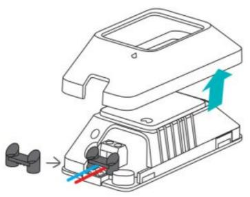
Remove the Protective cover, then connect wires before fixing the wire fastener.
