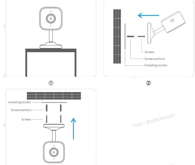
This device can be placed on a desktop (Figure ①), mounted on a wall (Figure ②), or installed on the ceiling (Figure ③).
