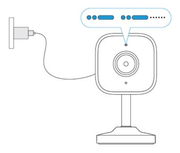
Insert the USB Type-C cable, once the device completes startup, it will enter the default pairing mode for the first use. The device LED indicator will then flash in a blue "short-short-long" pattern (if the LED indicator does not flash In this pattern, please press and hold the device reset button for 5 seconds to make the device enter the pairing mode again).
