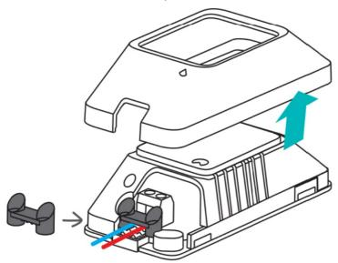
To make sure a full installation, please align " o " with " o " when securing the protective cover.
