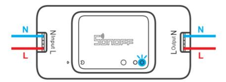
After powering on, the device will enter quick pairing mode (Touch) during the first use. The Wi-Fi LED indicator changes in a cycle of two short and one long flash and release.
