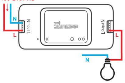
! Make sure the neutral wire and live wire connection is correct.
